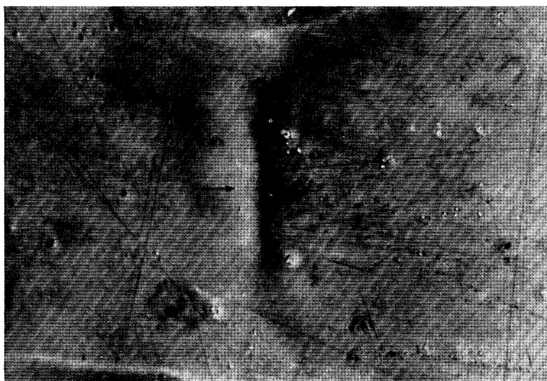
FIGURE 14. A small depression in copper. Depressions similar to this provide the first detectable signs of permanent deformation. The specimen illustrated has received 8000 impacts at 51 m/s. (Magn. \times 500 .) Phase contrast photograph.
