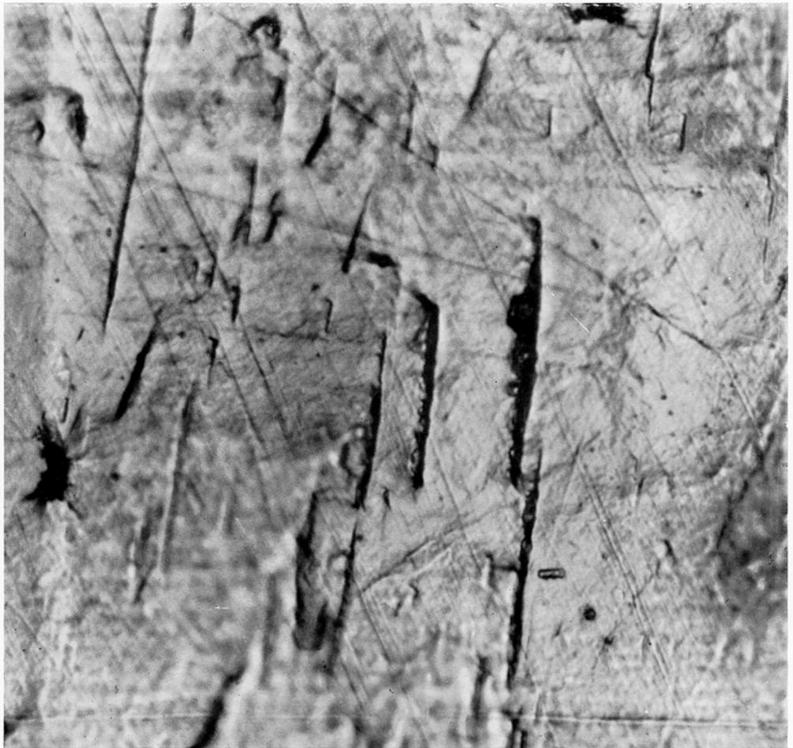
FIGURE 21. Shear deformation along twin boundaries in an iron single crystal. The centre of impact was to the right of the area photographed. 2.8 \times 10^5 impacts at 85 m/s. (Magn. \times 470 .)
